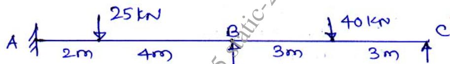
Q3) Analyze the beam by stiffness matrix method. Draw BMD.
